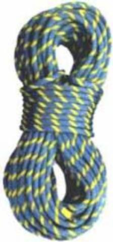
A modern climbing rope, a key piece of safety equipment, is of kernmantle construction, consisting of continuous braided nylon fibers, the kern, surrounded by a continuous braided nylon outer sheath, the mantle. Such construction is superior to the more traditional laid rope (three large strands twisted together) because the outer sheath protects the inner core, where most of the strength lies, from the elements.
