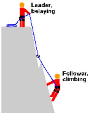
The leader's job is dangerous. Unlike top-roping, where slipping off the rock usually doesn't result in a long fall, a leader can fall twice the distance from the last piece of protection before the rope can help. The figure below depicts a fairly pleasant lead fall--the leader has fallen and is dangling in midair. More often, the leader will hit the rock on the way down--a common cause of climbing injuries.
