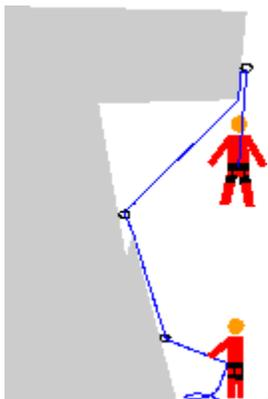
A "quickdraw"--two carabiners attached with a loop of webbing--is used to fasten the rope to a piece of protection. One carabiner is attached to the loop on the piece of protection, the rope is passed through the other. This provides some separation of protection a rope, allowing the rope to twist without dislodging the protection, pass more smoothly past the protection, and go more directly up the climb.
