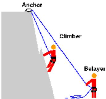
In top-roping, a rope from the top of the climb always holds the climber, making most slips off the climb harmless. As shown above, the climber is attached to one end of the rope, the middle is passed through an anchor at the top of the climb, and the other end is held by the belayer.
