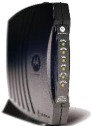
What exactly is a modem? Well it happens to be an Acronym for "**modulator-demodulator**". It is a device that modulates an analog carrier signal to encode digital information, and also demodulates such a carrier signal to decode the transmitted information. The goal is to produce a signal that can be transmitted easily and decoded to reproduce the original digital data. Modems can be used over any means of transmitting analog signals, from driven diodes to radio.
